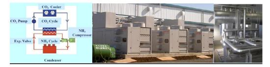
The principle scheme shows the CO2 secondary brine circuit(in blue color) and the NH3 compressor circuit (in red color).
