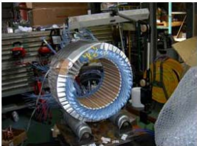
Building the stator
