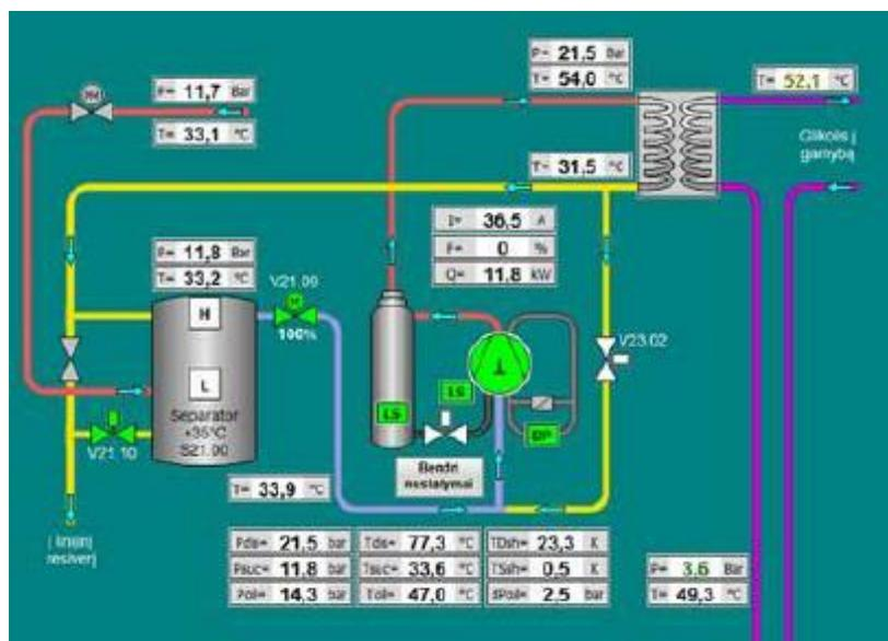
Figure 3. hot water NH3 heat pump
