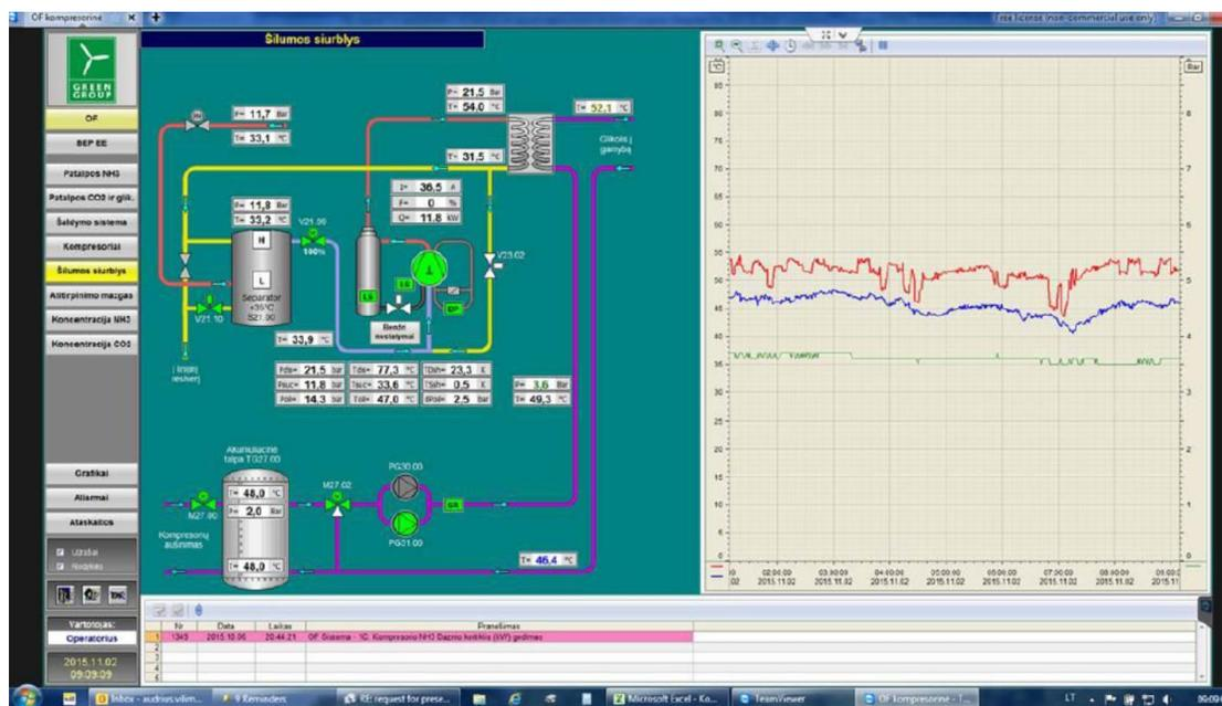
Figure 7. heat pump system & trend supervision
