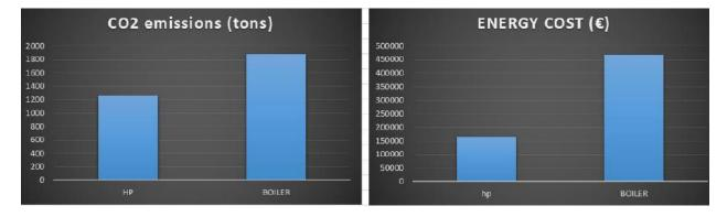
The investment for the heat pump amount to 400.000 €, while it is only 50.000 € in case of the gasboiler. The maintenance cost over a period of 15 years has been estimated at 400.000 € for the heat pumps. Calculating the investment and the energy costs for a 15 years operation period results in 3.370.490 € for the heat pump, while 7.056.560 € for the gas boiler or a saving of 3.686.070 € for the heat pump solution.
